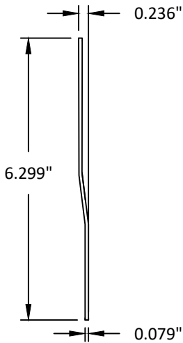
6 INSTALLATION FIN CARBON GALVANIZED STEEL
